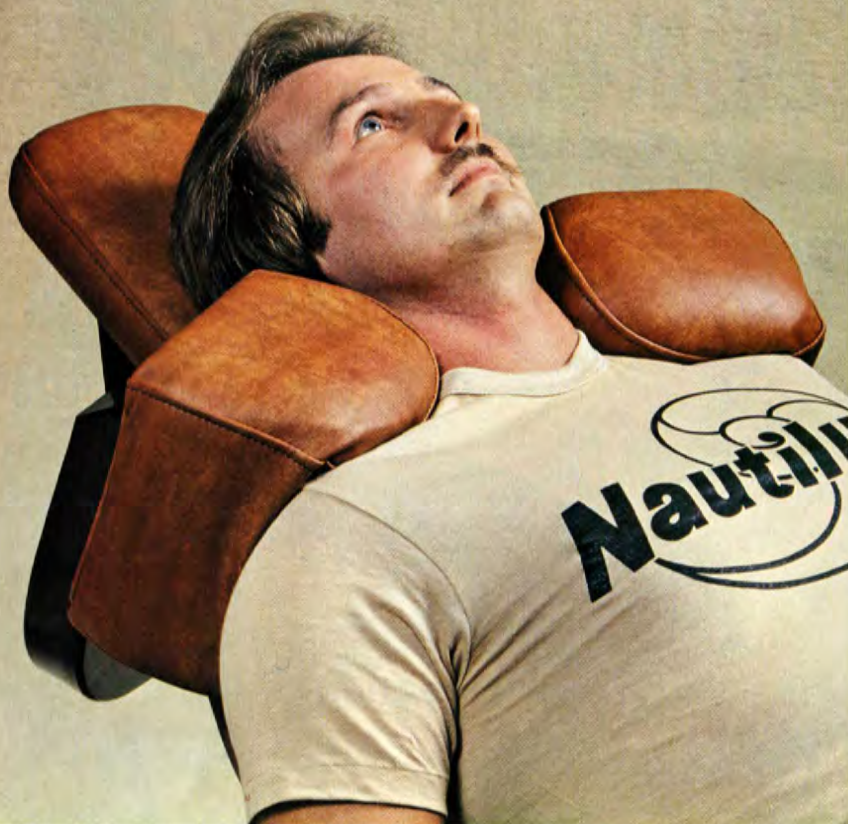
The head and shoulder pads on the Duo Squat machine. The shoulder pads are made of soft, solid foam, brush cut and formed to fit the contours of the shoulders for comfort.
